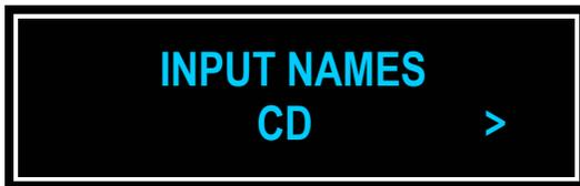
3. The first Input on the list is CD. Press the **▶RIGHT** button twice to scroll to UNBALANCED 2.
