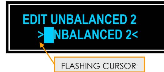
5. Each character may be changed by scrolling through the available character list using the **▲UP** and **▼DOWN** Buttons. When the desired character is reached, move the cursor using the **◀LEFT** or **▶RIGHT** Buttons to change another.
