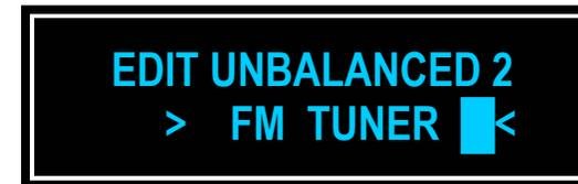
6. Press **•ENTER** to save temporarily. The display will return to that of Step 3. The user may go on to edit other Input names or exit the menu system by pressing **▲UP** to retreat through the menu structure.
