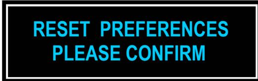
6. Press ● **ENTER** to CONFIRM the RESET to previously saved user settings. The Menu will automatically be exited.
